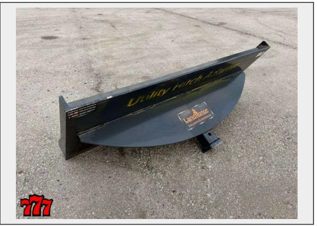
**Description** 10" depth, 3000lbs max lift capacity. **Quantity:** 1
